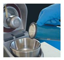
Mortar and pestle made of chrome steel or stainless steel are deep frozen with liquid nitrogen.
